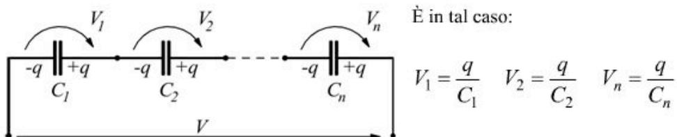
$$V = V_1 + V_2 + \dots + V_n = \frac{q}{C_1} + \frac{q}{C_2} + \dots + \frac{q}{C_n} = q \cdot \left( \frac{1}{C_1} + \frac{1}{C_2} + \dots + \frac{1}{C_n} \right)$$
