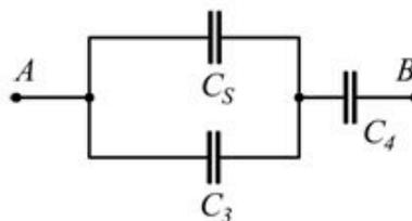
$$C_S = \frac{1}{\frac{1}{C_1} + \frac{1}{C_2}} = \frac{1}{\frac{1}{160 \cdot 10^{-12}} + \frac{1}{200 \cdot 10^{-12}}} = 88,9 \text{ pF}$$
